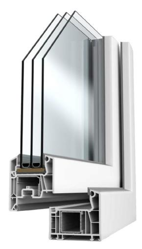
The configuration of the fold with a depth of 28 mm makes possible glazing from 18 mm to 48 mm (depending on the rod used).
